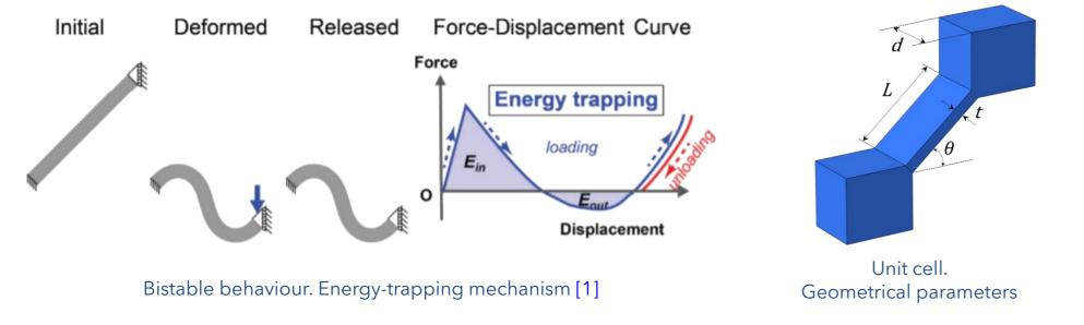
1.1. Polydimethylsiloxane (PDMS): The material considered in the analysis is PDMS, an elastomeric material valid for its use in additive manufacturing processes, a technology that offers a convenient method for rapidly fabricating materials composed of arrays of tilted elastic beams in programmable motifs.
