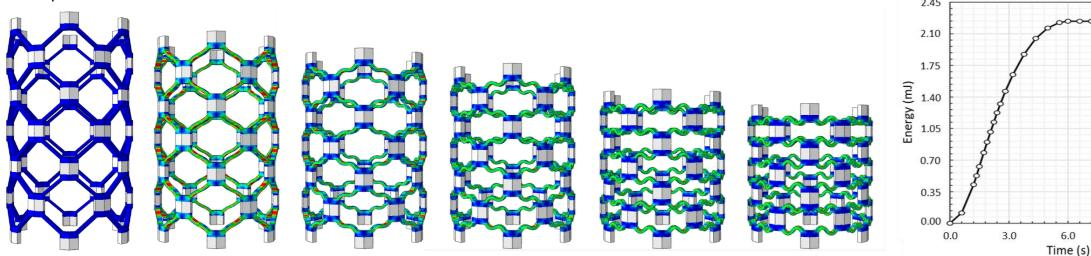
3.2. Dynamic behavior: In this case, it is possible to observe the different time instants which the collapse of each of the levels of the cylindrical metastructure takes place in. It is also interesting that the successive collapses do not always occur between contiguous heights because of the influence of the wave propagation phenomena.
